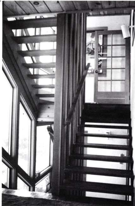
6, 7, Lee-Carmichael house. The solar collector is here a staircase which acts like a greenhouse from which heat is circulated to the surrounding 'thin-mass' room.
