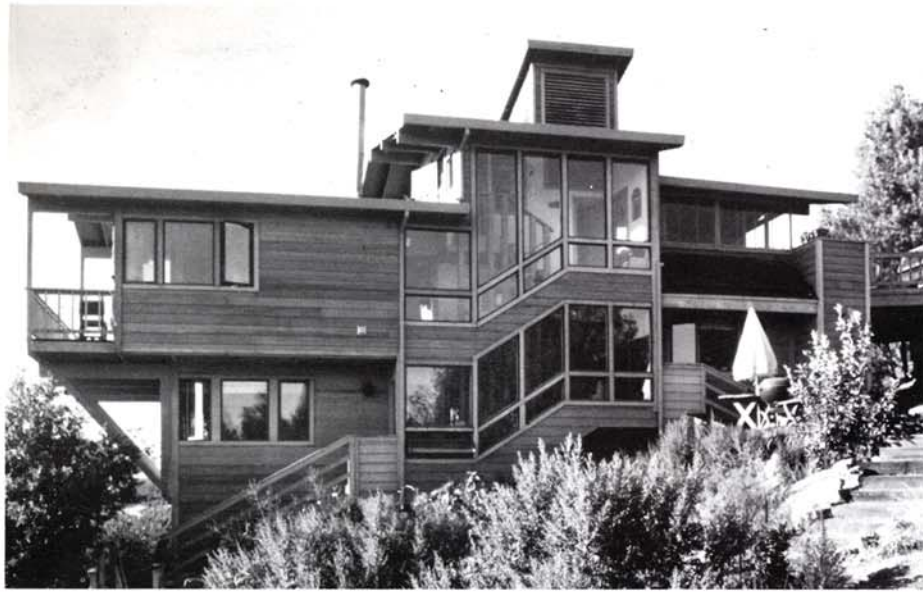
6, 7, Lee-Carmichael house. The solar collector is here a staircase which acts like a greenhouse from which heat is circulated to the surrounding 'thin-mass' room.
