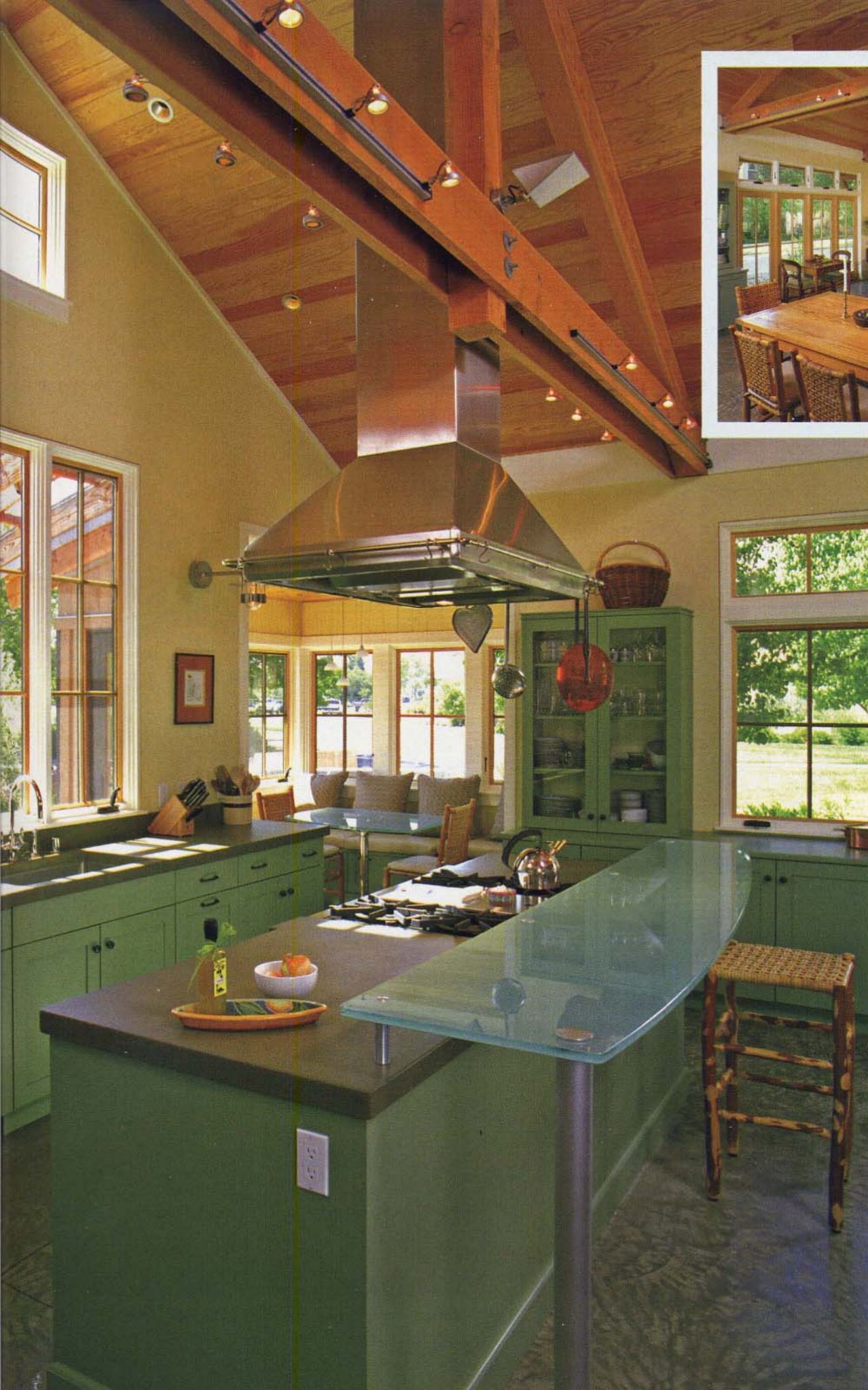
Natural light from four sides. Simple trusses and a wood ceiling emphasize the territorial style in the great room. Windows and sliding doors on all four walls ensure plenty of light and cross ventilation. Burnished concrete floors help to moderate indoor temperatures. Photo taken at C on floor plan.
